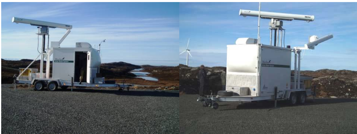
Figure 1. The Merlin Avian Radar System that gather data on Smøla. Photo: Roel May ©
